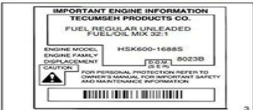
Tecumseh engine model, specification, and D.O.M. number are now located on a decal adhered to the blower housing.
