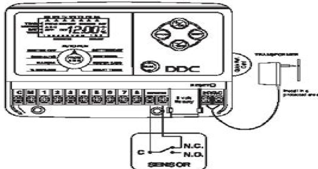
To connect a rain sensor, remove the jumper wire from the sensor terminals and connect one wire of the Toro Rain Switch to the 'C-common' terminal and the other wire to the N.O. (normally closed) terminal. As soon as the Rain Switch contacts change from the N.C. position to the N.O. (normally open) position, irrigation will be suspended. Irrigation will resume as soon as the Rain Switch closes and its contacts return to the N.C. position.
