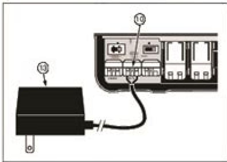
2. Connect one transformer cable wire to each terminal labeled 24 VAC (10). The wires can be connected to either terminal.
