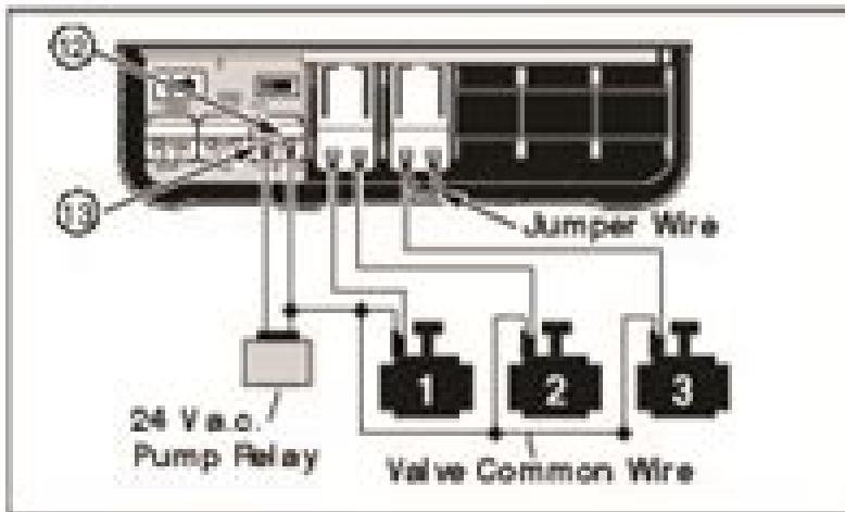
**CAUTION:** To prevent pump damage due to "dead-heading," connect a jumper wire from any unused zone terminal to a zone terminal with a valve connected.
