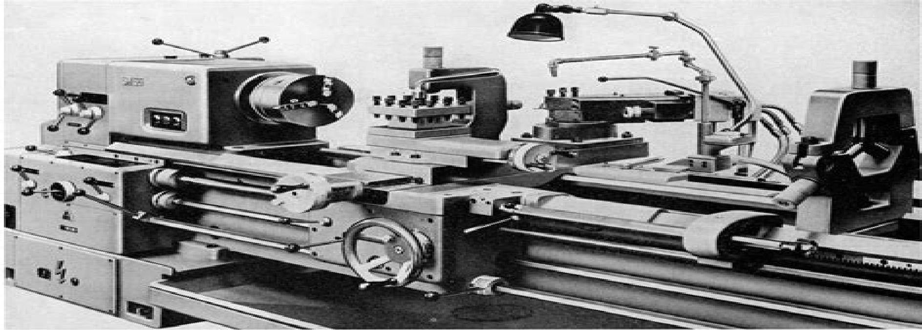
**SN 55 lathe with follow rest and steady rest**
