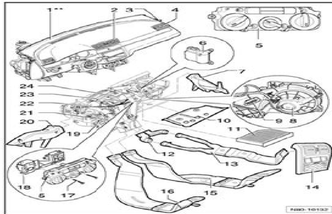
Disconnect battery before removing components marked with \*\*
