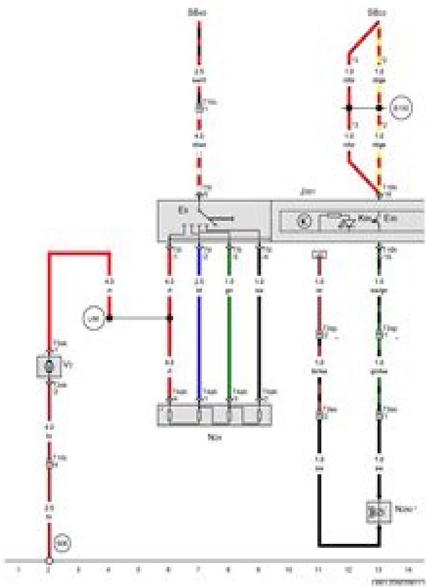
Fresh air blower switch, Air conditioning system control unit, Fresh air blower series resistor with overheatng fuse, Fresh air blower
