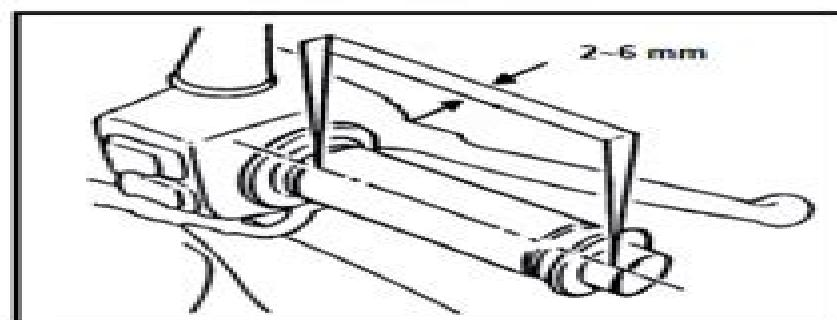
Adjustment can be done in either ends. Secondary adjustment is conducted from top side.
