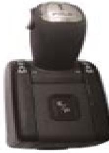
This gear lever can be folded forward when the vehicle is at a standstill, placed alongside the seat cushion so it is not in the way when the driver wants to move around.
