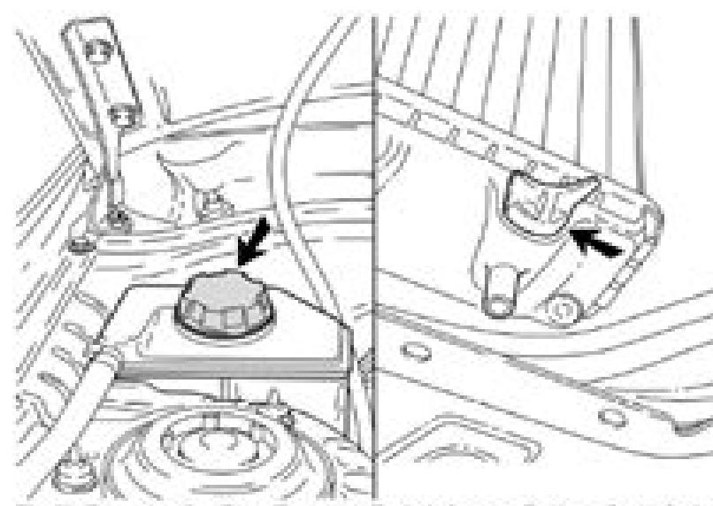
Fig. 11- Removing Cap From Expansion Tank & Opening Radiator Drain Cock
