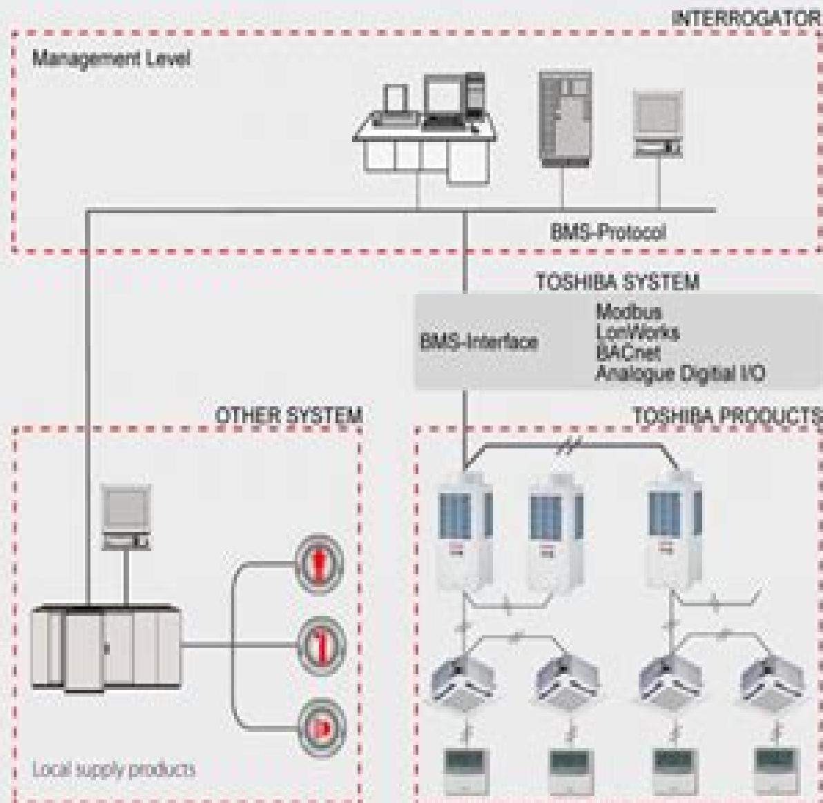
BMS interface products are not compatible with each other across protocols. Only one protocol can be used per installation.
