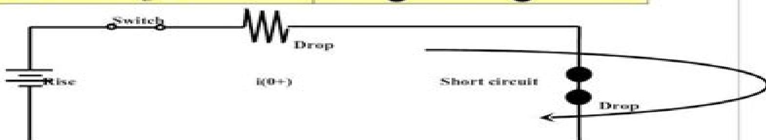
Applying KVL for  $t \geq 0$
