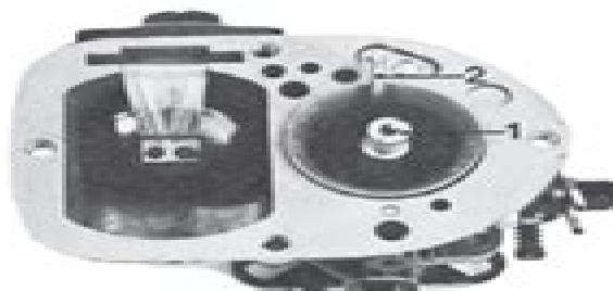
3. Lift out the float and check it for leakage. Should the float leak, the float level will not be correct. The weight of the float should be 7.3 grams (0.26 oz's). Remove the emulsion jet (1) and the acceleration jet (2).
