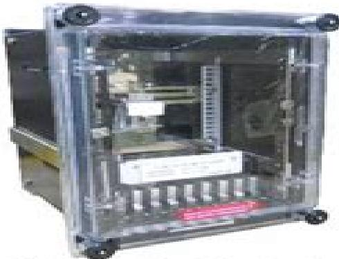
VAPM31 Relay is used for detection of failure or inadvertent removal of voltage transformer secondary fuses and for prevention of incorrect tripping of circuit breakers.
