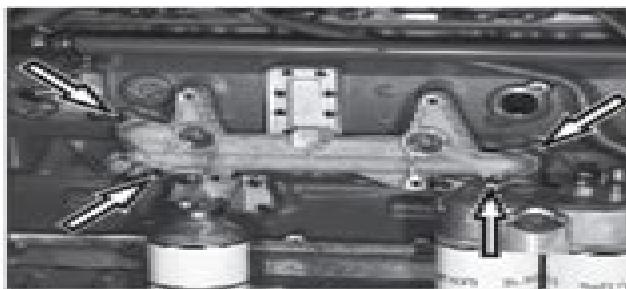
Remove the spacer plate (four screws).
