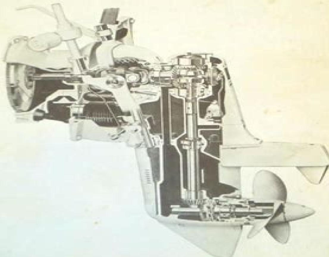
**OUTBOARD DRIVE UNIT MODELS B and C**
