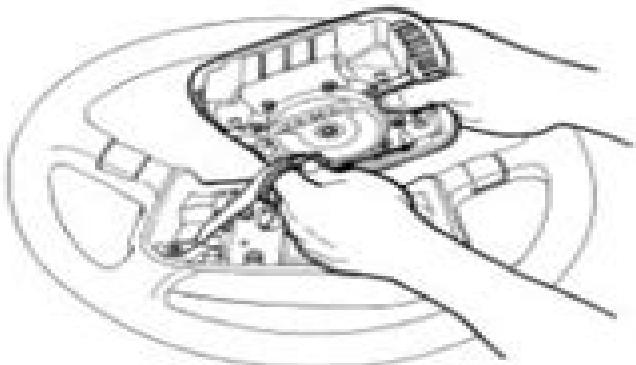
Disconnect the airbag module electrical connector and remove the airbag module.
