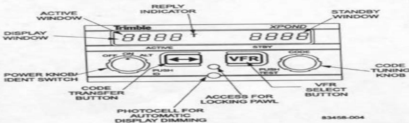
The active code is displayed on the left side of the display window and the standby code is displayed on the right side. The transponder displays a "T" (reply indicator) to the right of the active code when it responds to an interrogation from a ground station indicating that the aircraft is being seen on radar. The "T" also verifies proper operation when using the self-test feature.
