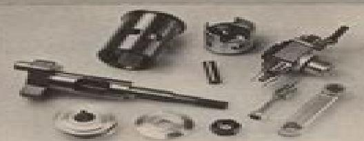
Crank has 17mm main journal. Ringed piston runs in Schnuerle-ported steel liner.
