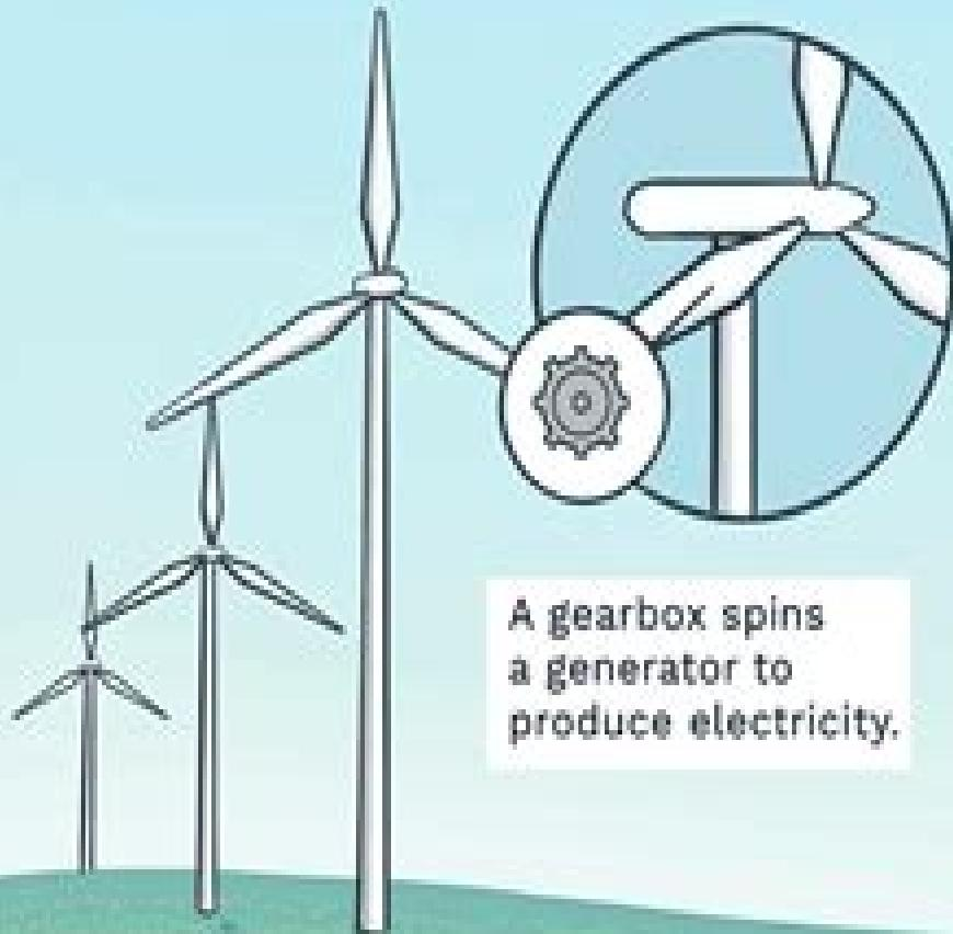
A gearbox spins a generator to produce electricity.
