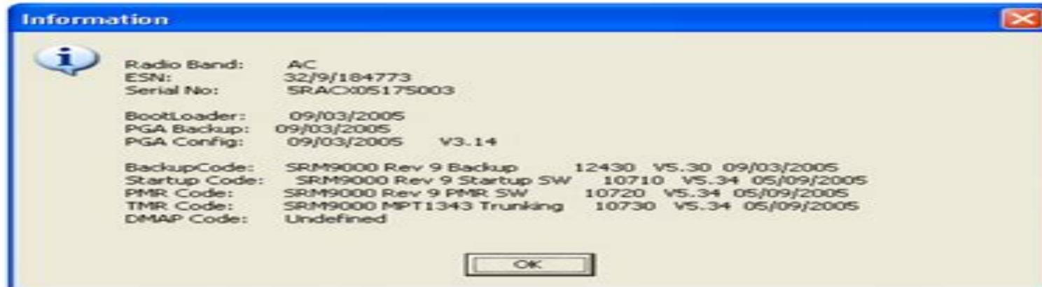
**SRM9030 Control Head SW** can be displayed on the Control Head by holding the '3' button down when the radio is switched on. This is only implemented in CH V1.06 SW (Oct/2000) and later.
