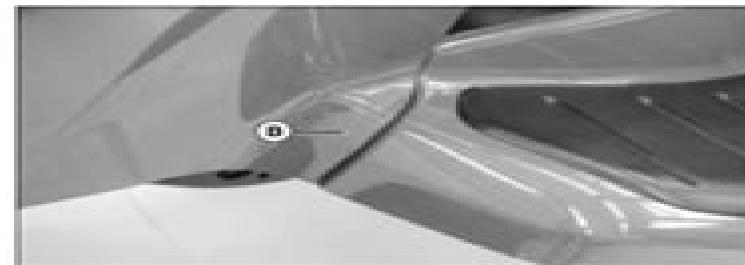
2. Check to be sure hood tabs (B) catch in frame on both sides of machine.
