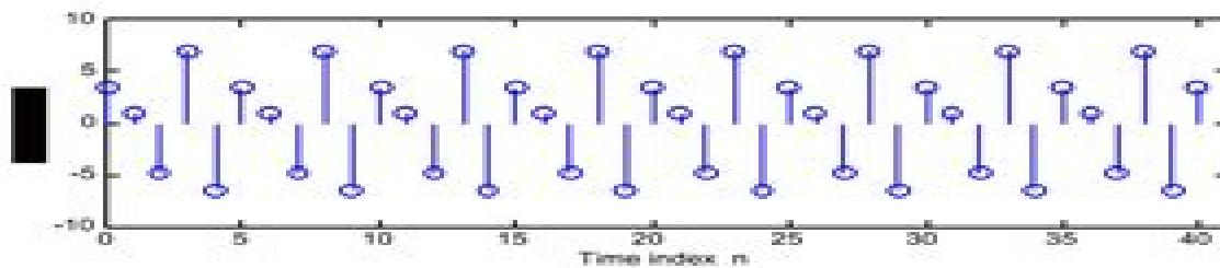
(b) Code fragment used to generate  $x_6[n] = n \bmod 6$  is: `x = rem(n, 6)`
