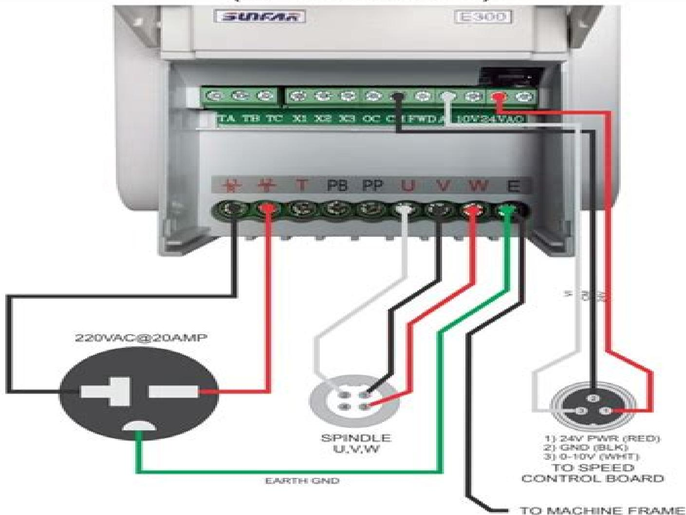
**NOTICE:** Internal wiring of Chinese spindles is not consistent. If spindle spins in reverse, swap U & V. You **MUST** verify visually or physically the proper rotation of the spindle to ensure the machine cuts properly!
