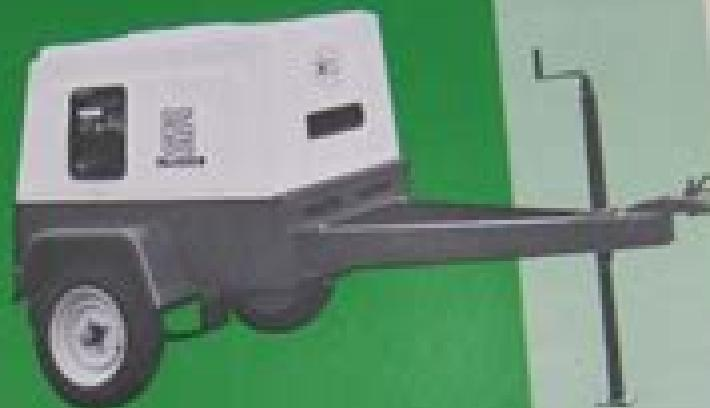
Compact Rotary Screw Air Compressor
