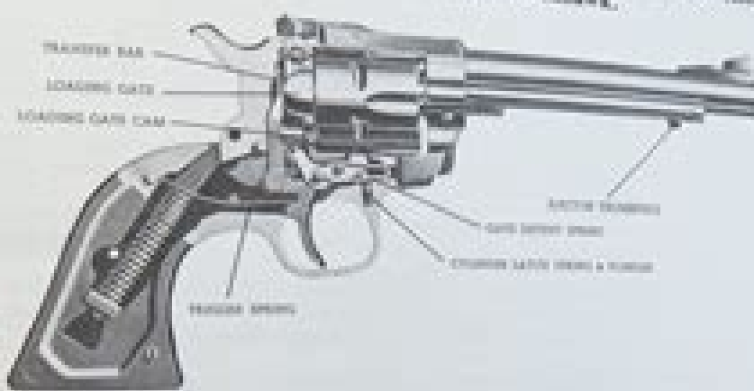
Mechanism shown at rest. Transfer bar is not in line between hammer and firing pin. This is the carrying position.
