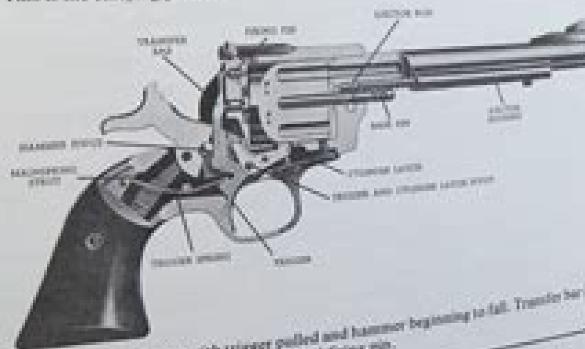
Mechanism shown with trigger pulled and hammer beginning to fall. Transfer bar is in firing position, between hammer and firing pin.
