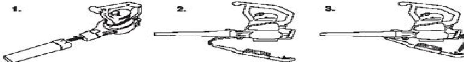
Important: You must install the blower tube before installing the inlet cover because the inlet cover hooks onto the blower tube. The blower will not run unless the bottom inlet cover is locked in place.
