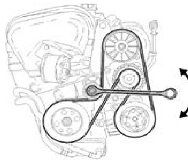
**Fig. 14: Removing/Installing Drive Belt**
