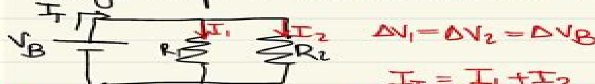
$$R_T = \frac{1}{\frac{1}{R_1} + \frac{1}{R_2} + \dots}$$
