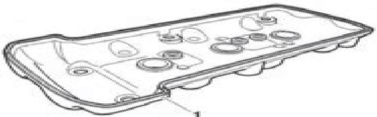
1. Camshaft cover seal groove.
