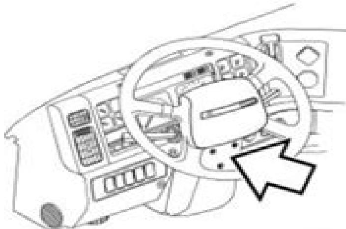
Remove the rear steering column cover by removing the 3 torx bolts from the cover and sliding the rubber
