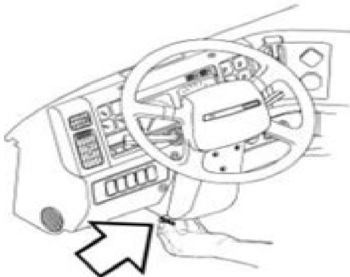
Remove the 2 clips at the bottom of the steering column cover.
