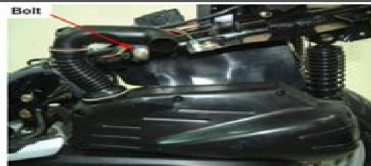
Remove 6 screws, and then remove the air cleaner element.
