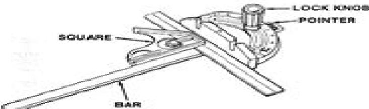
2. Position the head square with the bar . . . tighten the lock knob.
