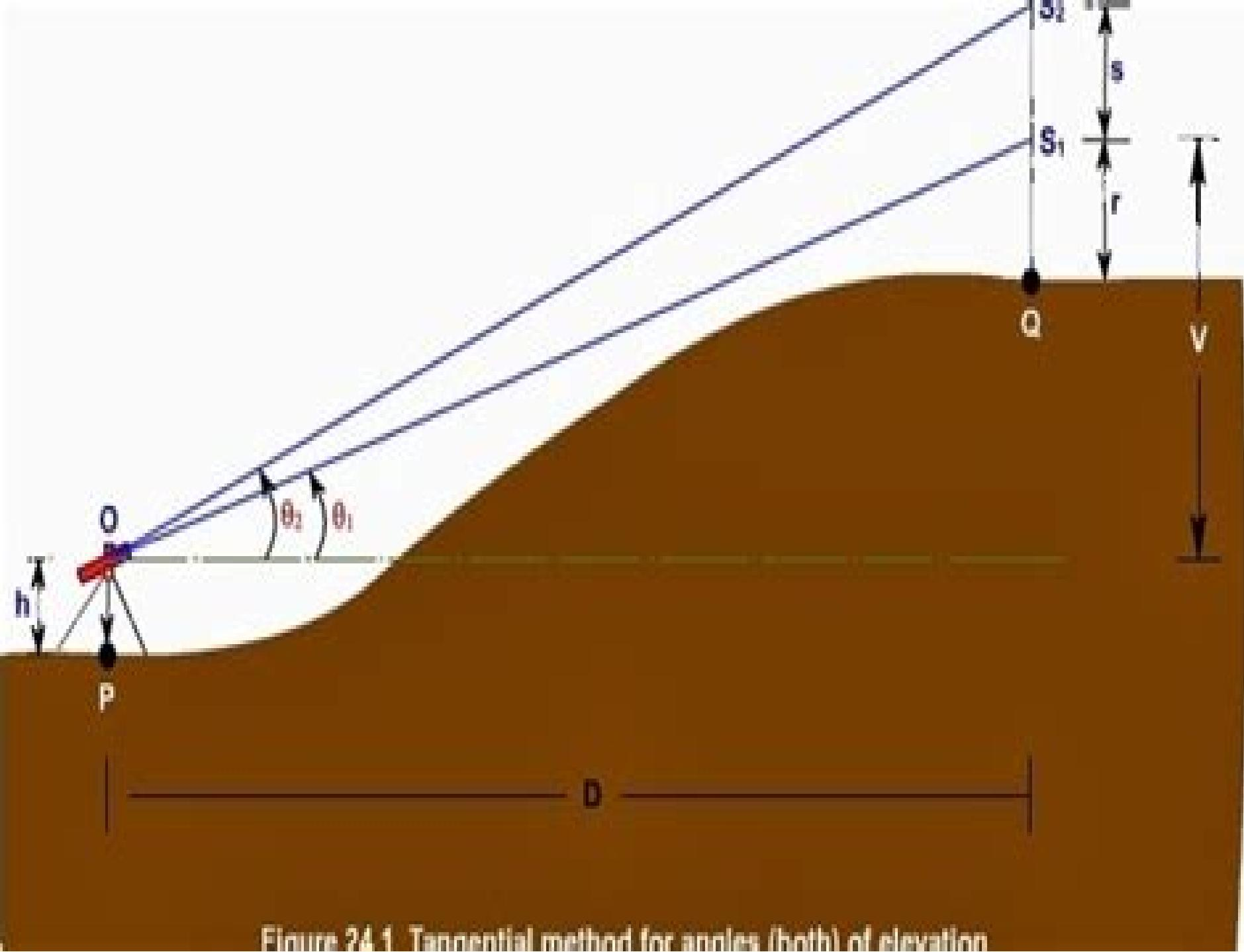
Figure 24.1. Tangential method for angles (both) of elevation
