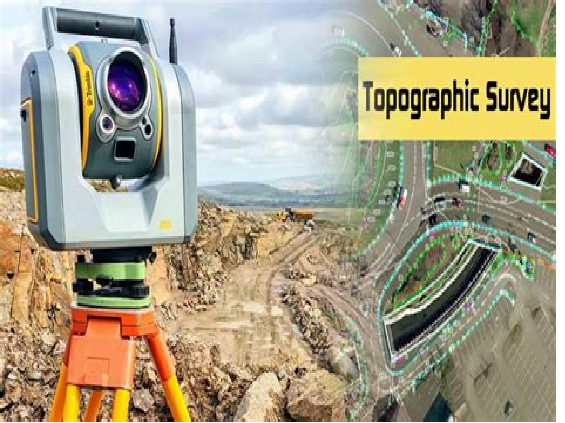
A composite image illustrating topographic surveying. On the left, a total station is mounted on an orange tripod, pointing towards a construction site with a bulldozer. On the right, a digital tablet displays a 3D topographic map of the same site, showing terrain elevation and survey points. A yellow banner with the text "Topographic Survey" is overlaid on the map.
