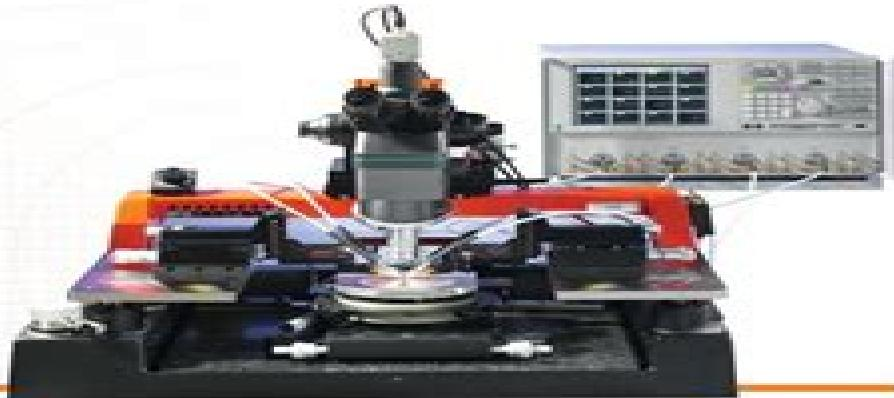
The PM8 is the ideal solution for precise analytical probing applications up to 200 mm including device and wafer characterization, failure analysis (FA), RF, mm-wave, sub-THz, optoelectronic-engineering and MEMS. The PM8 is designed specifically to provide a highly stable, ergonomic and flexible probing platform.
