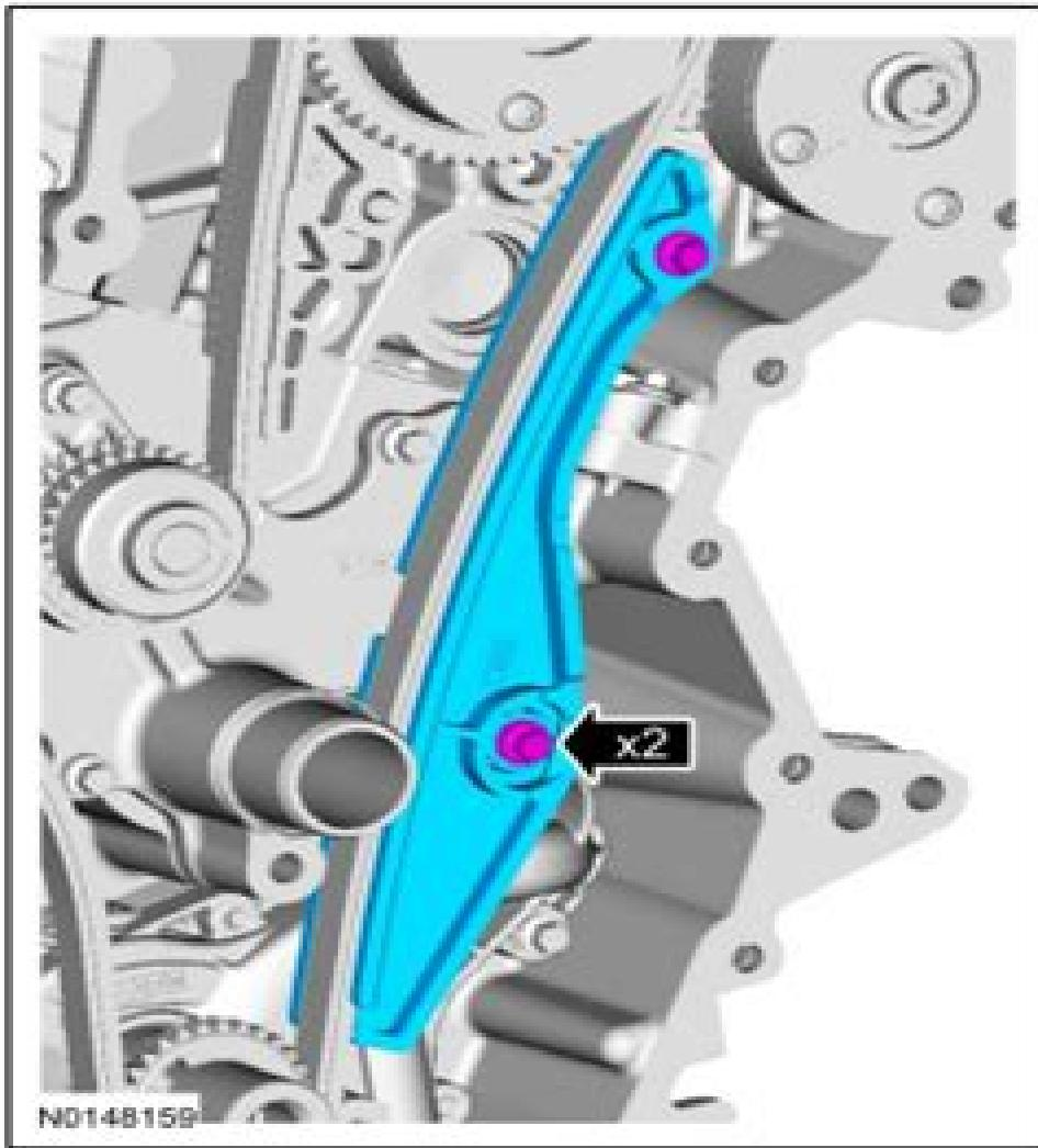
99. Install the primary timing chain tensioner arm.
