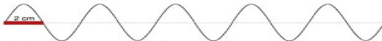
a) How many waves are there in this wave train? 5b) Wavelength 4 cm c) Amplitude 2 cm d) frequency 5 Hz e) speed 20 cm/s**Wave 2**
