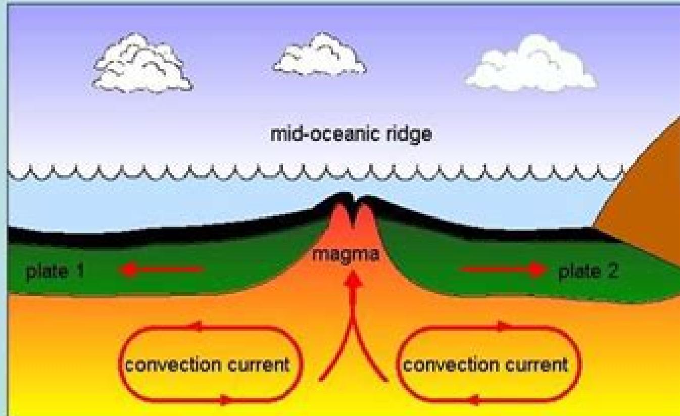
Plate 1 and plate 2 move apart. Magma rises, cools and solidifies forming new igneous rock. This is sea-floor spreading and is a constructive plate boundary.
