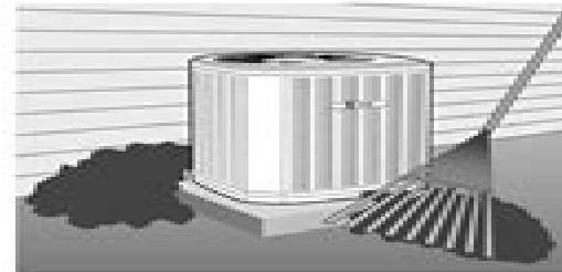
Efficiency can be maintained by keeping outdoor unit clear of debris, leaves and shrubbery.
