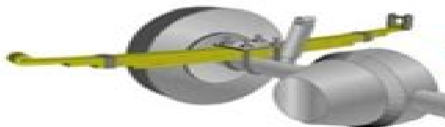
Left: Solid axle rear suspension with leaf springs. Right: Solid axle "trailing arm" rear suspension for a front-wheel-drive model. Note the track bar directly above the axle.
