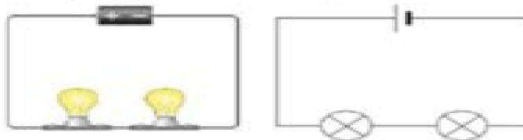
If you put more lamps into a series circuit, the lamps will be dimmer than before.
