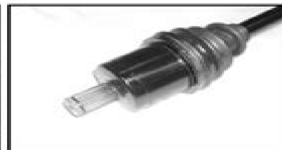
Figure 14-6 Compression Ring on Spline
