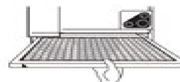
Slide dirty filter out, replace with a new filter making sure the arrows printed on it are pointing in the direction of airflow.
