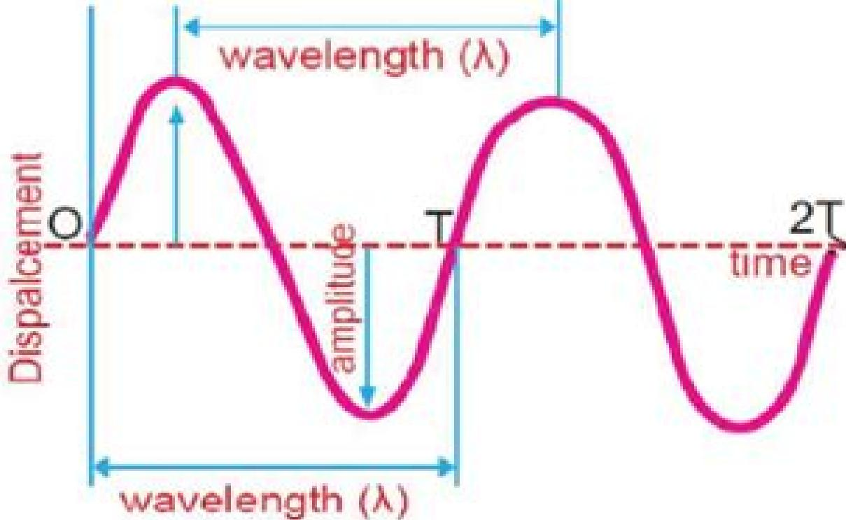
The *frequency* is related to the period and has units of Hz, or  $s^{-1}$ . The number of such oscillations per unit time is the frequency of the sound wave.  $\nu = \frac{1}{T}$
