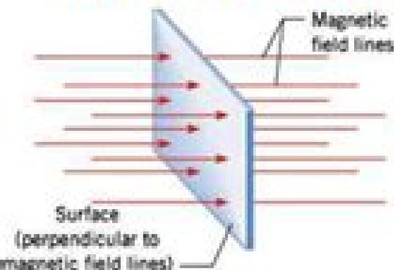
The magnetic flux is proportional to the number of field lines that passthrough a surface.
