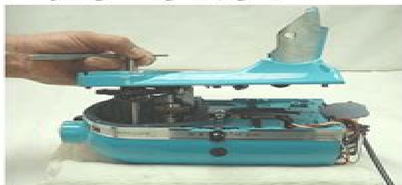
Fig. 60 Initial mating of bottom cover to gearcase - motor housing.
