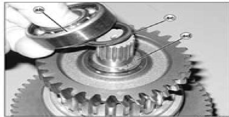
17. Remove bearing (ab), washer (ac), and snap ring (ad).
