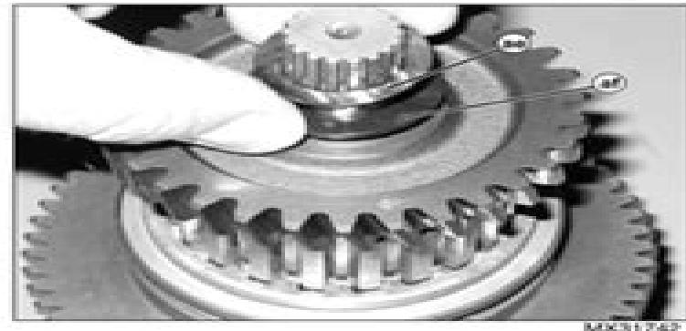
18. Remove washer (ac) and thrust washer (ad).
