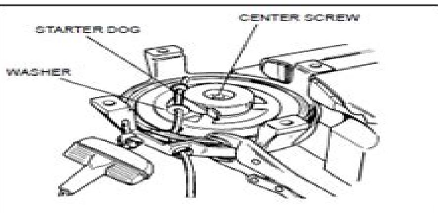
Turn the center screw clockwise to center the starter hub containing the starter dogs in the center cup so there is equal contact on all the dogs into the teeth of the cup.
