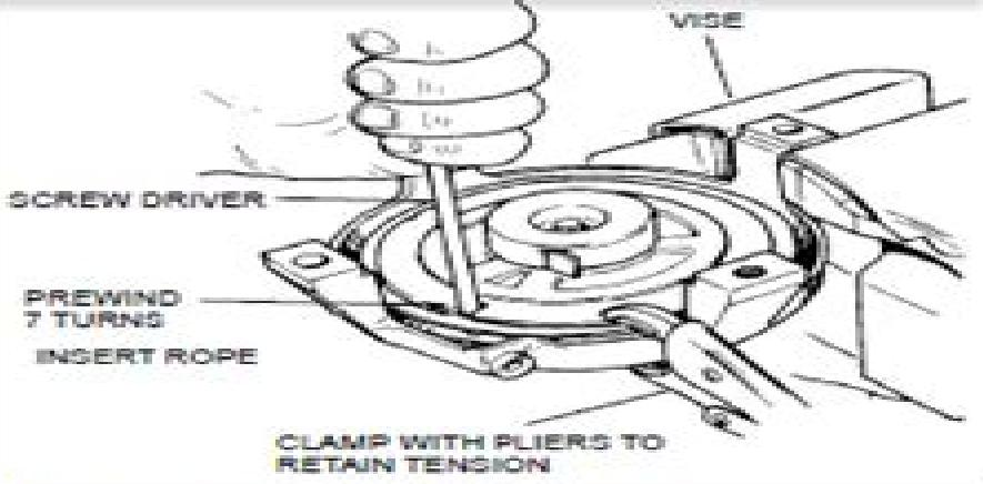
**ROPE REPLACEMENT.** Prepare the rope, place a thin 3/4" (19.05 mm) diameter washer with a 1/4" (3.175 mm) hole on the rope and tie a knot. The other end of the rope should be thinned to a point for easier threading.
