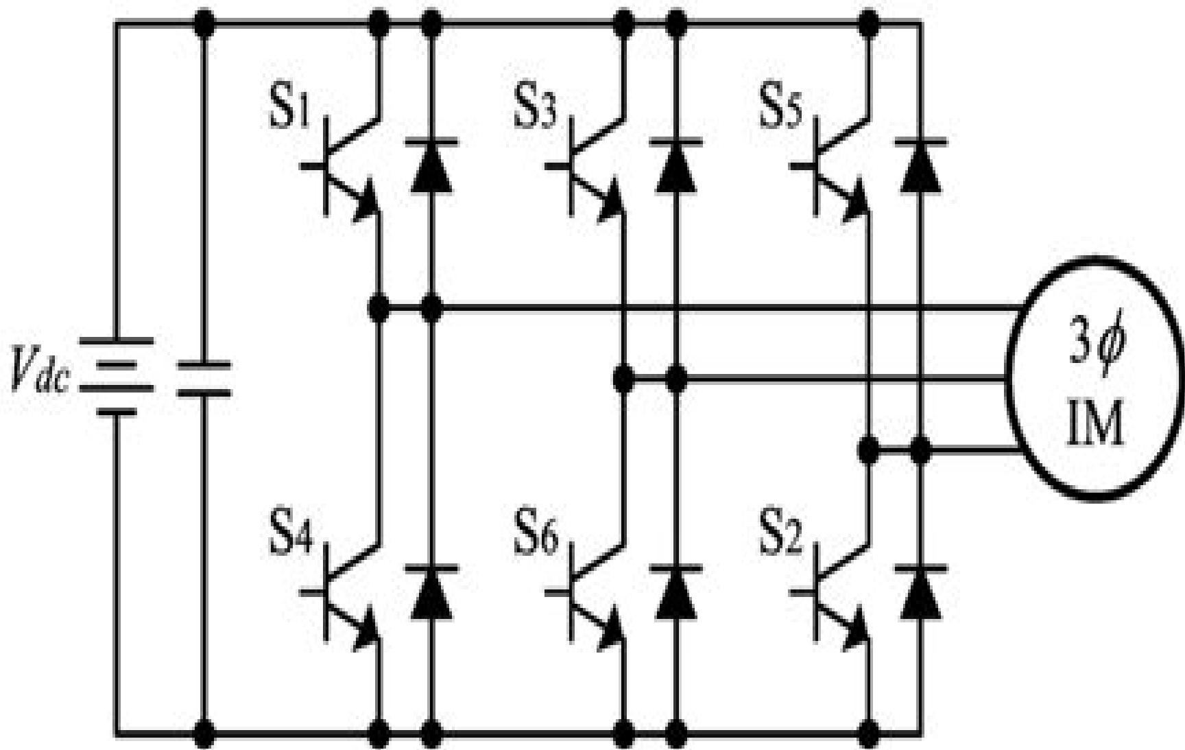
Three Phase Inverter Circuit
