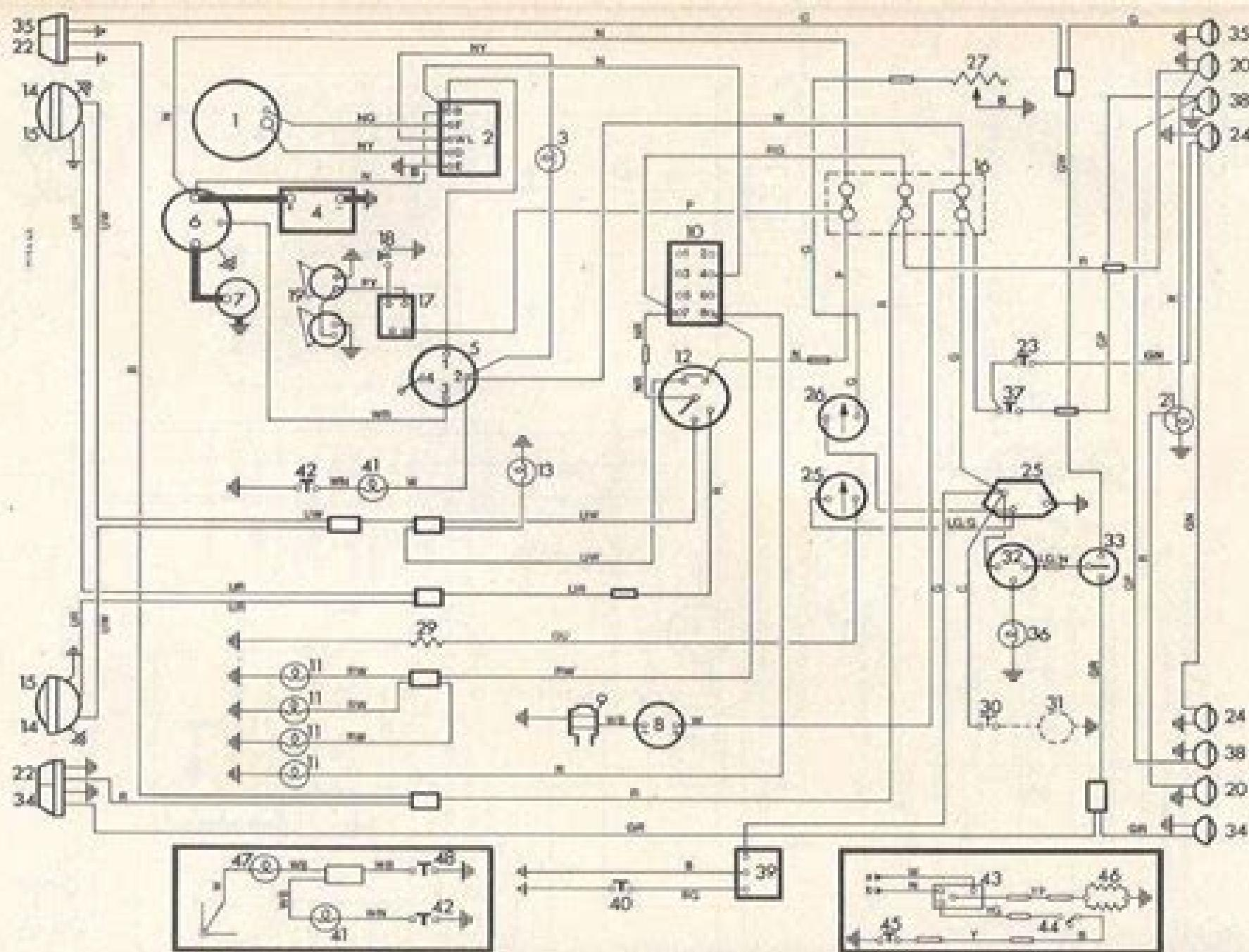
Fig. 10.54 Wiring diagram for Spitfire Mk. III negative earth RHD and LHD
